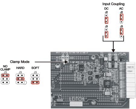
Figure 7-2. Coupling and Clamp Configuration Options
